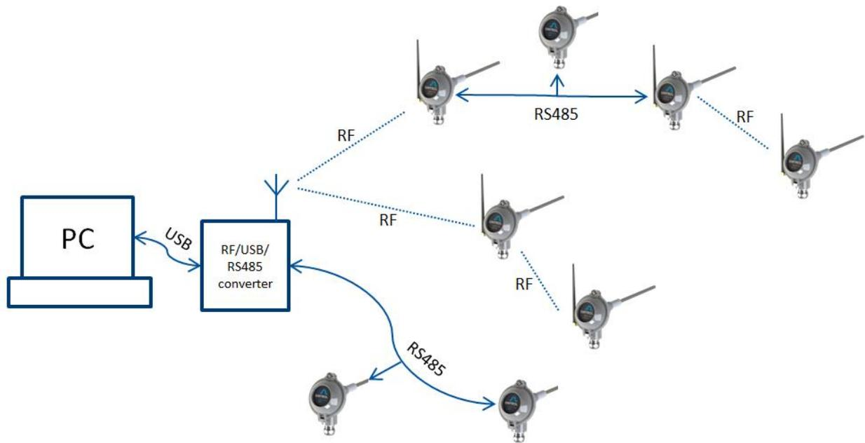
Figure 9 Sintrol Network topology
