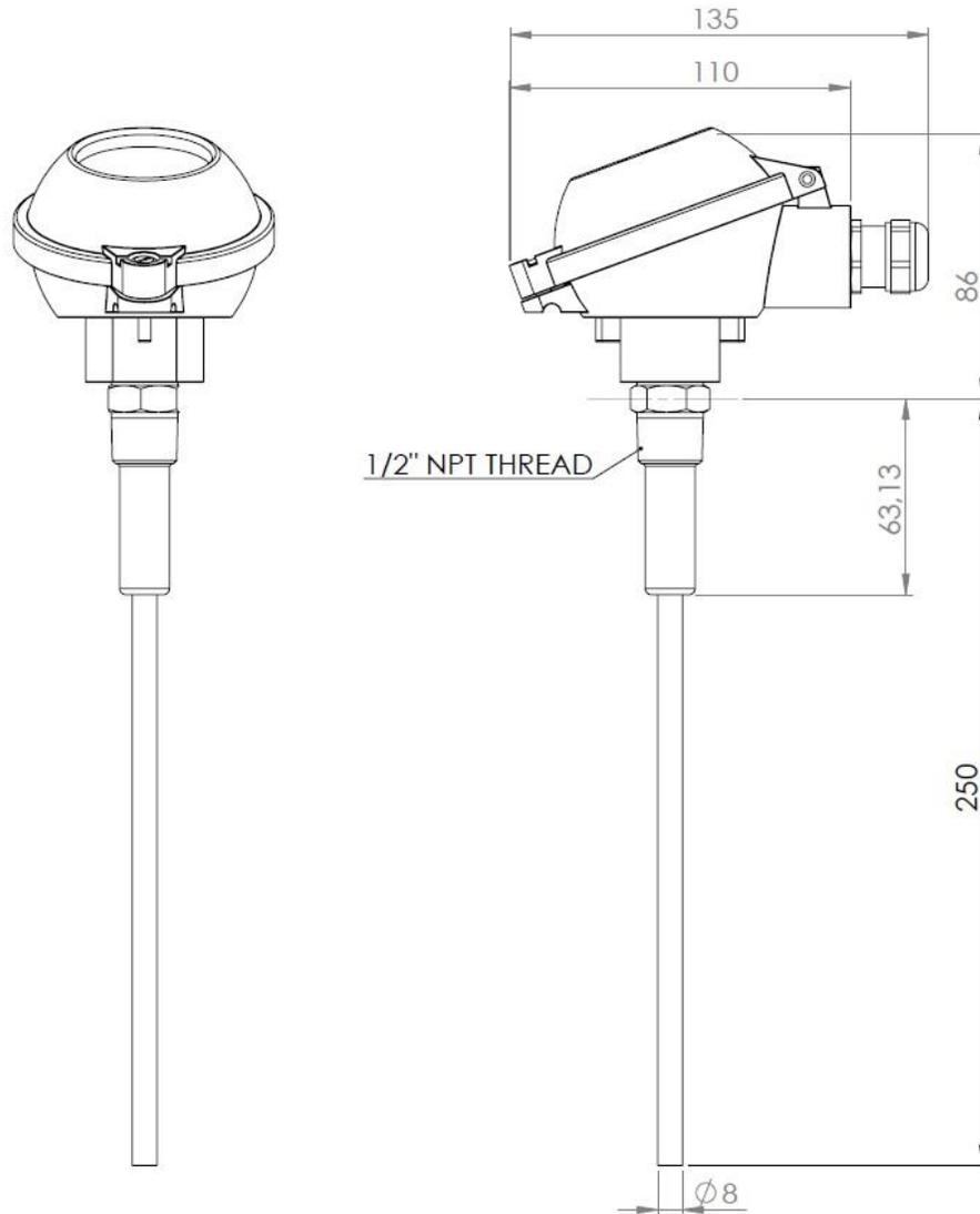
**Figure 4 Structure and dimensions**
